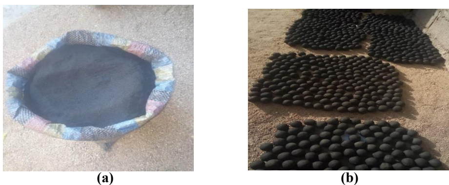
Figure 8: (a) Coal powder obtained after carbonization and crushing of the raw material;
