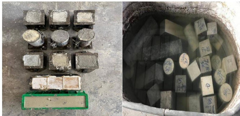
Figure 3 a) Casting b) Curing of SIFCON .
