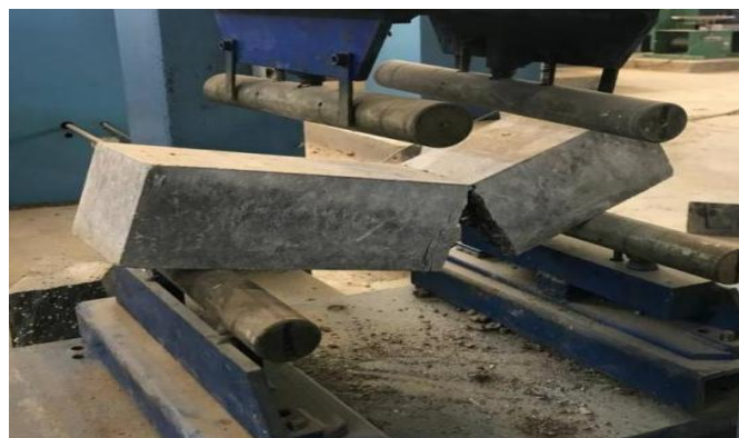
Figure 7. Flexural strength test was carried out in Mustansiriyah university, college of engineering
