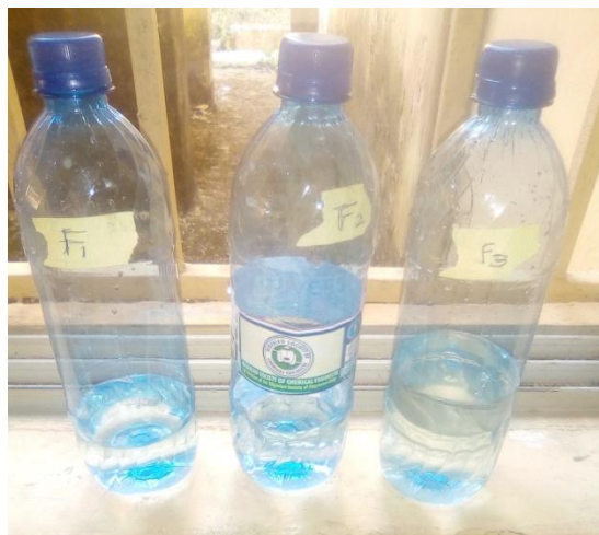
Figure 3 Appearance of the water after filtration through the ceramic water filters
