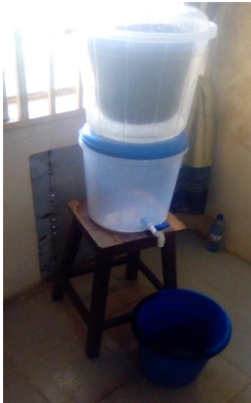
Figure 2 Ceramic water filter put in the 15 litres bucket and connected to the storage tank
