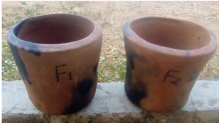
Figure 1 Conical frustum-shaped ceramic water filter
